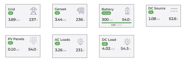
**Source** and **Load** are the different convention signs used for the different assets. The conventions of the different assets are listed in the below table. Based on the type of asset, the widget icon is displayed on the home page.
