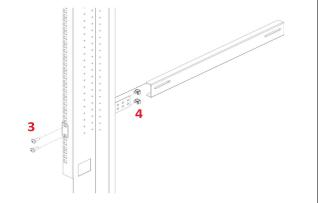
Assemble the sliders and adjust the length to suit the mounting depth.
