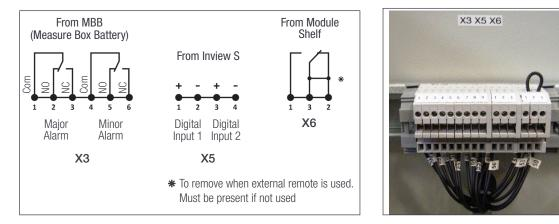
When an alarm occurs, the X3 relay contacts are de-energized and switch.
