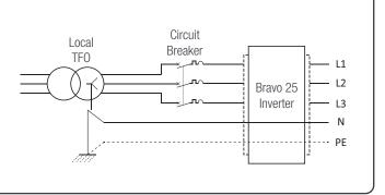
The AC input is wired to a screw terminal. Max cable area is 180 mm<sup>2</sup>
